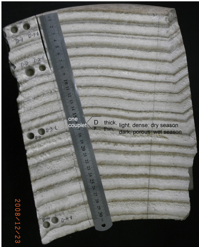
Fig. 8. Section of the sampled travertine near the spring S1-1. Visible is the alternation of thin dark porous warm-rainy-season layers and thick light dense cold-dry-season layers. A couplet comprising a thin and a thick layer represents one annual cycle.
