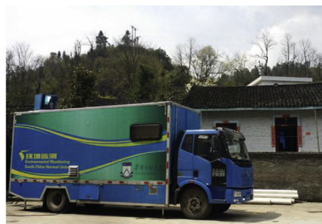
Fig. 1. The South China Normal University mobile system operating on site in Wanshan for monitoring of atmospheric atomic mercury.
