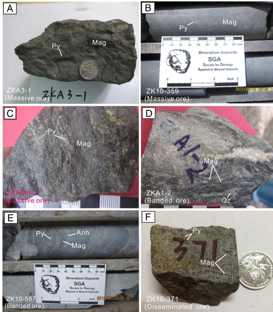
Fig. 4. Photographs of ores from the Zankan Fe deposit. (A) Massive ore containing magnetite and pyrite; (B), (C) Massive ore containing magnetite and laminated pyrite; (D) Banded ore containing magnetite, and quartz; (E) Banded ore containing magnetite, laminated pyrite and anhydrite; (F) Disseminated ore containing magnetite and pyrite. Abbreviations: Mag, magnetite; Py, pyrite; Qz, quartz; Anh, anhydrite.
