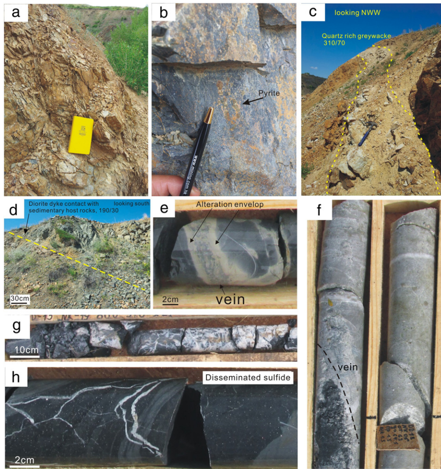
Fig. 4. a. high angle schistosity in metasedimentary host rocks in the mine pit. The orange and brown colors are due to oxidation; b. trace of fine-grained pyrite in the metasedimentary host rocks; c. quartz-rich greywacke layer in a metasedimentary unit. NWW-SEE strike with steep bedding; d. N-S oriented diorite dyke within a metasedimentary unit; e. restricted alteration envelopes surrounding veins in carbonaceous wall rock. Alteration is characterized by bleaching to pale greenish/ grey colour; f. pervasive alteration in greywacke surrounding auriferous vein, including predominantly silicification, sericite, carbonate alteration; g. quartz-carbonate breccia vein with high gold grade, composed of wall rocks fragments cemented by quartz; h. disseminated sulfides in host black shale.
