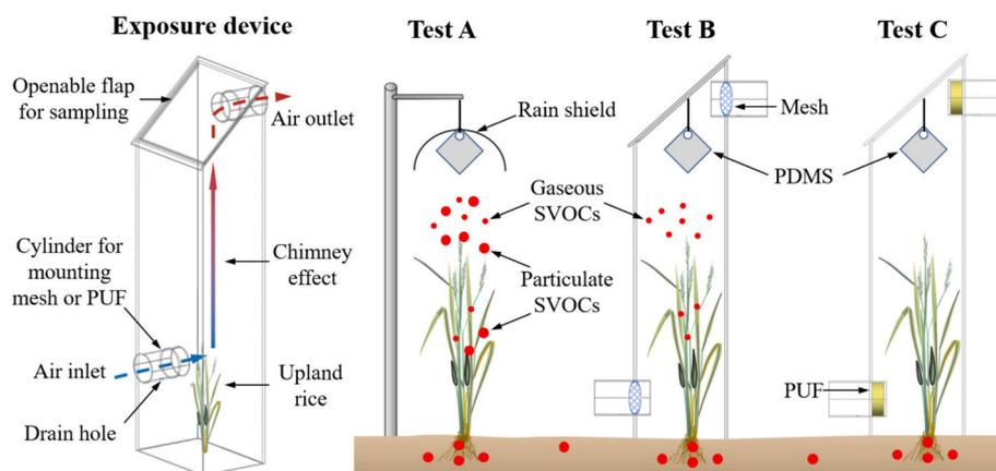
Fig. 1. Specific exposure devices and field exposure experiments of upland rice to OPEs, PAEs, and PAHs via soil, gas, and particle uptake pathways.
