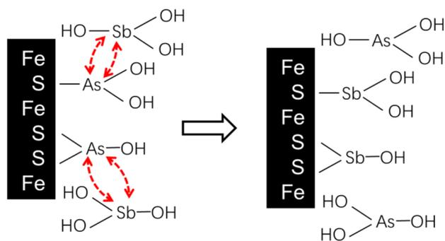
**Fig. 4** Proposed reaction for the competition of As(III) and Sb(III) on the surface of FeS at pH 7.0
