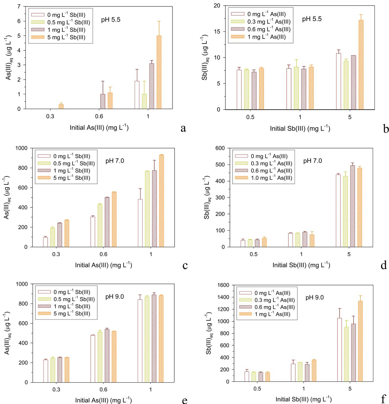
**Fig. 1** Residual As(III)<sub>aq</sub> and Sb(III)<sub>aq</sub> concentrations in the treatments in which As(III) and Sb(III) were simultaneously added (FeS: 44 mg L<sup>-1</sup>; reaction time: 24 h)
