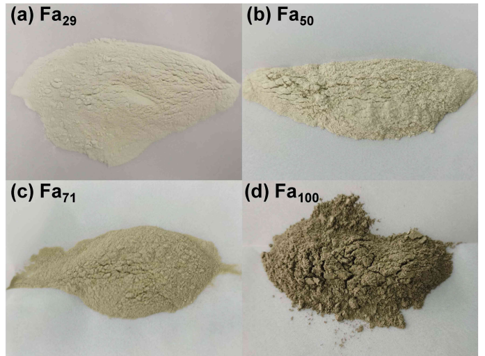
Fig. A.3. Synthetic Fe-rich olivine powders before laser irradiation. The grain size of the powders is <75 μm. Image (a) Fa 29 , (b) Fa 50 , (c) Fa 71 , and (d) Fa 100 . The colors of the initial olivine gradually change from white to dark green with increasing Fe content.
