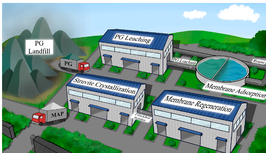
Fig. 1. Schematic illustration of the integrated membrane-triggered adsorption combining struvite crystallization concept for phosphorus recovery from PG leachate.
