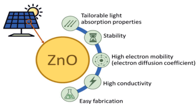
Fig. 4. The diagram illustrates the primary benefits and characteristics of ZnO semiconductor materials for solar cells and photo-catalysis applications.
