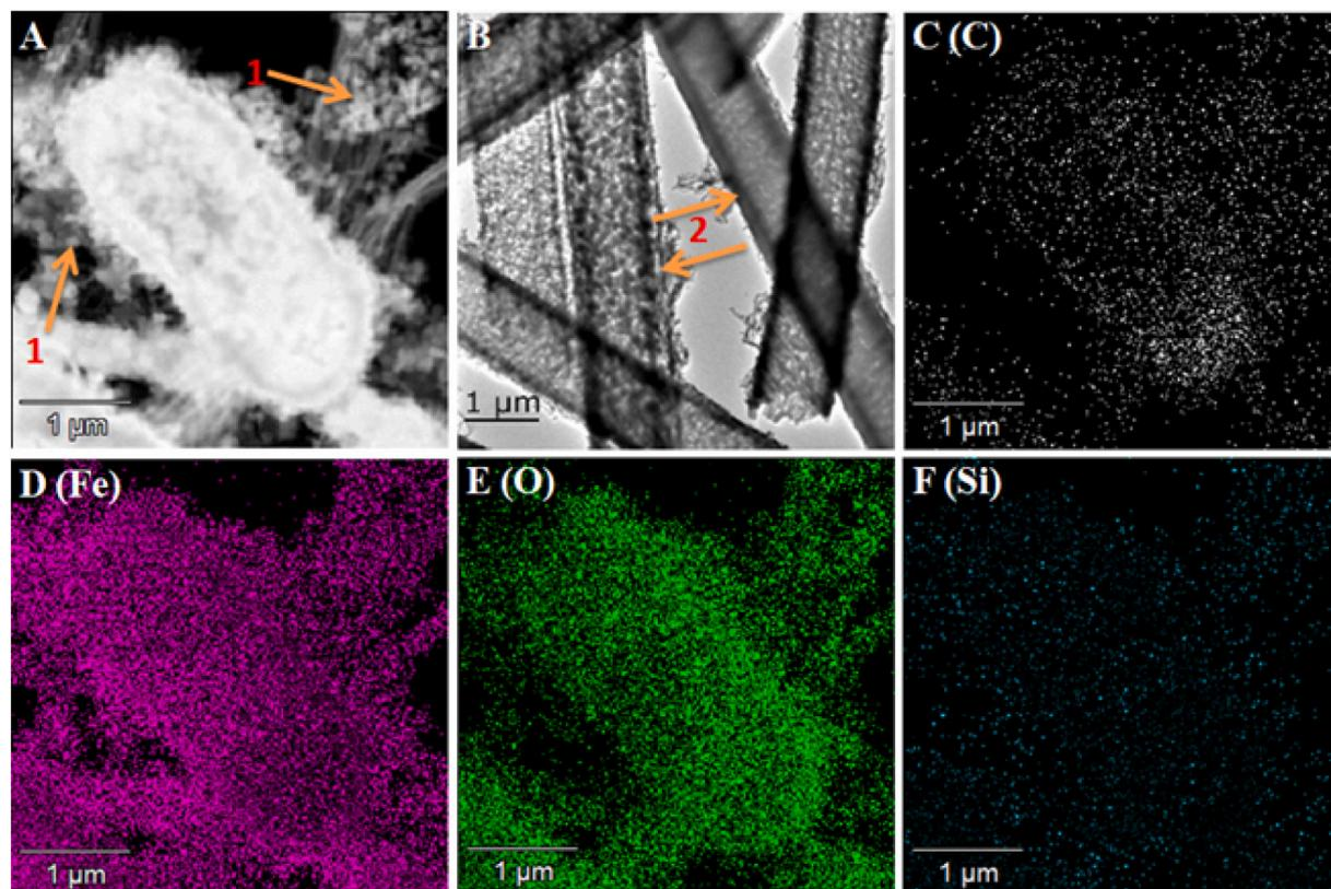
**Fig. 2.** The TEM image of floating Fe films (A-B) with disorganized Fe-oxyhydroxide particulates (1) and sheaths morphologies (2). The EDS mapping of floating Fe films shows carbon, Fe, oxygen, and silicon distributions in micrographs (C-F).
