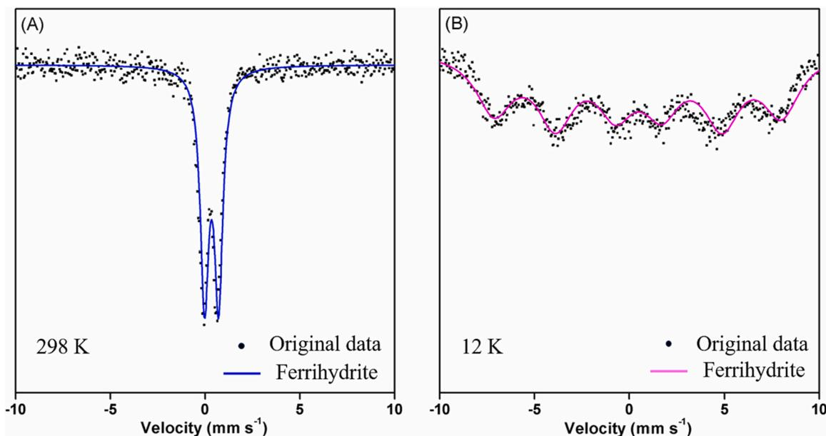
Fig. 1. Fitted Mössbauer spectra of floating Fe films at (A) 298 K and (B) 12 K. The circles represent the original data, and the solid lines represent the fitted curves. Corresponding fit parameters are summarized in Table S1.
