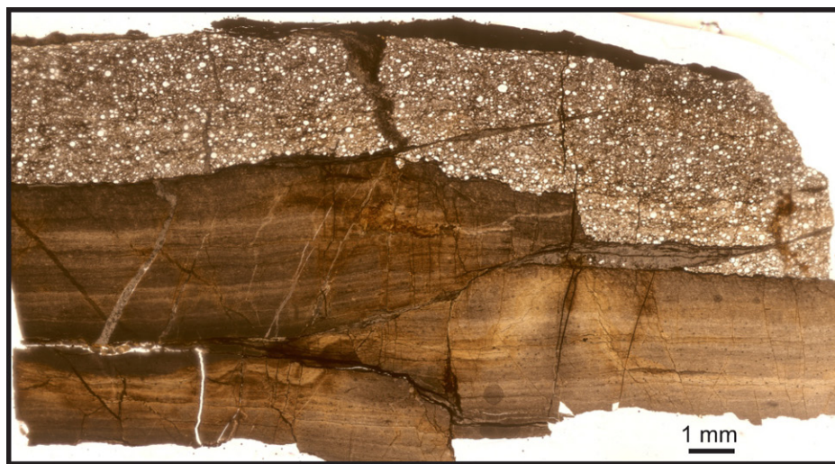
Figure 3. Thin-section photograph showing finely laminated siliceous mudstone below and radiolarian-rich level above (4.0 m stratigraphic height at Island Bay, Waiheke Island, New Zealand; Fig. 2). Small fractures offset lamination to a minor extent.
