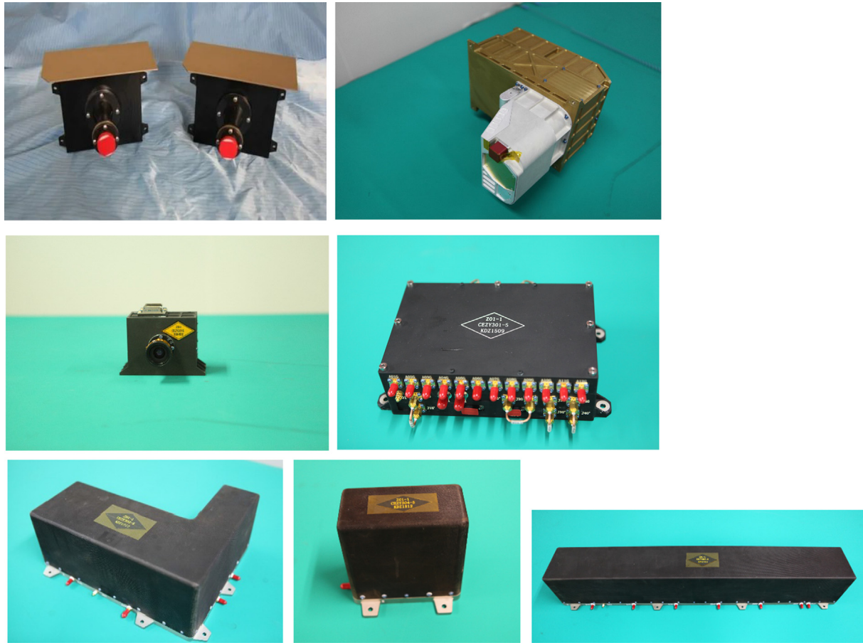
Fig. 7. The scientific payloads (from left to right, first row: Panoramic Camera, Lunar Mineralogical Spectrometer, second row: Landing Camera, Lunar Regolith Penetrating Radar Controller, third row: Antenna of Lunar Regolith Penetrating Radar A/B/C).
