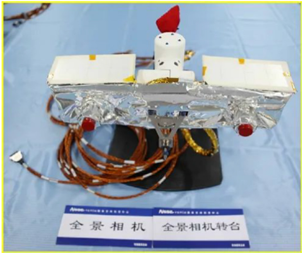
Fig. 10. Assembly picture of panoramic camera and rotating mechanism (range of rotating mechanism: azimuth angle: -90° to +90°, pitch angle: -85° to +90°).
