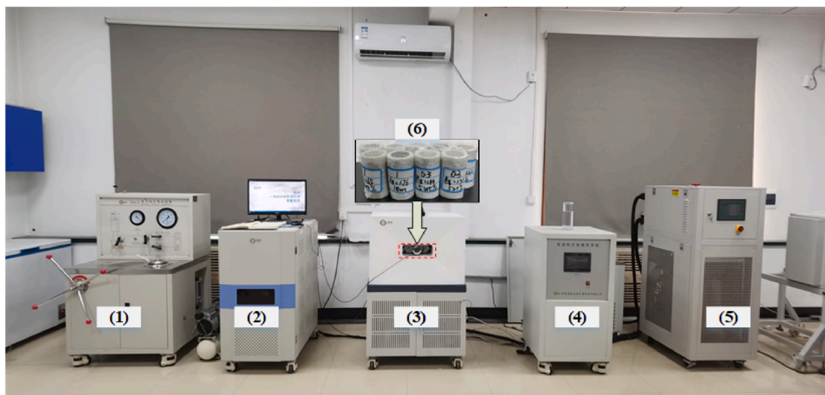
Fig. 2. MesoMR12-060H-I medium-size MRI analyzer (1) vacuum pressurized saturation unit; (2) industrial control machine; (3) magnet cabinet; (4) low-temperature heat exchange circulation system; (5) refrigeration heating circulation unit; (6) samples used in the test.
