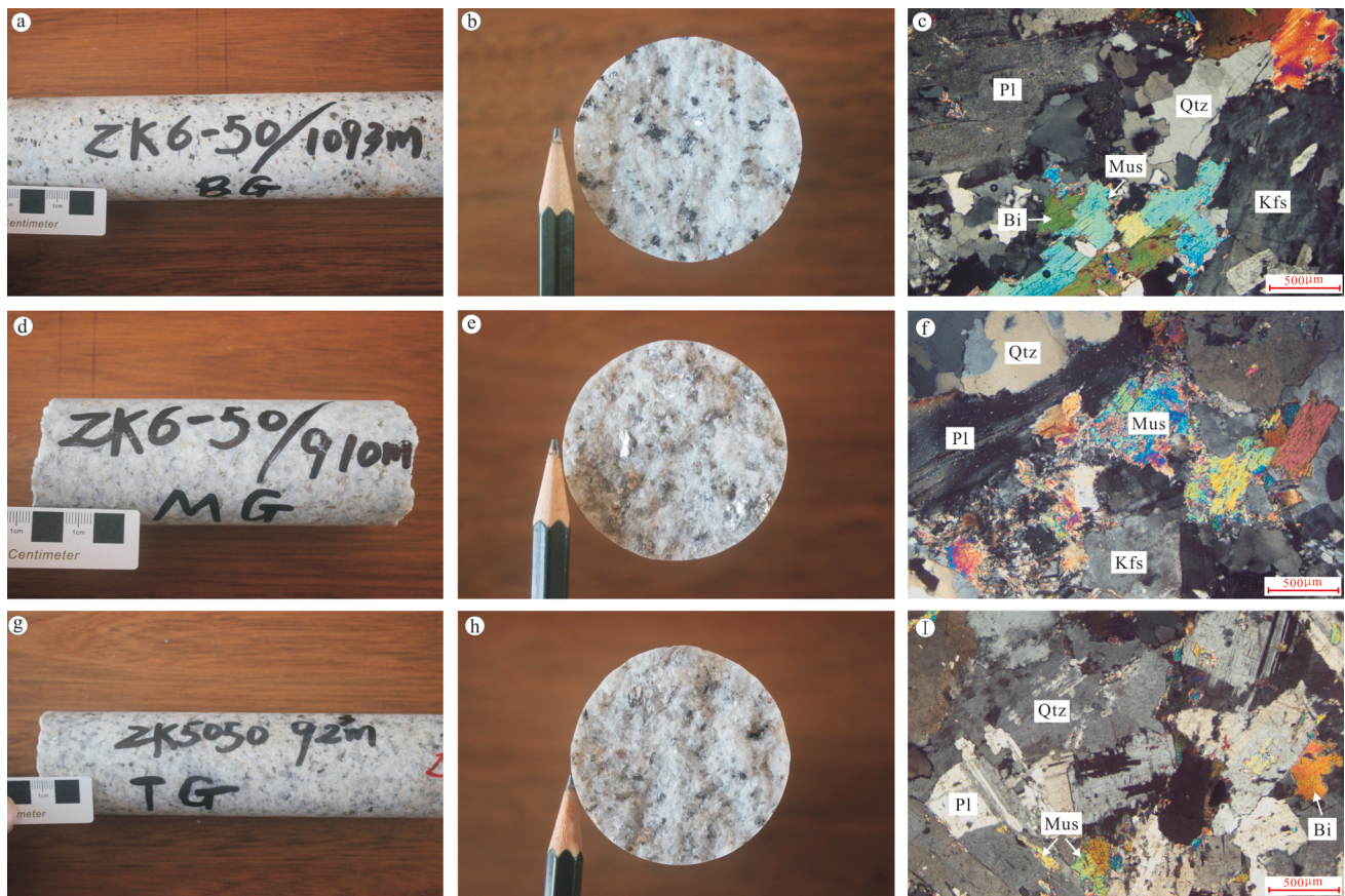
Fig. 3. Photographs of granite samples from the Dongping W deposit. (a–b) medium-grained biotite granite (sample DPBG); (c–d) medium-grained muscovite granite (sample DPMG); (e–f) medium-grained two-mica granite (sample DPTG).
