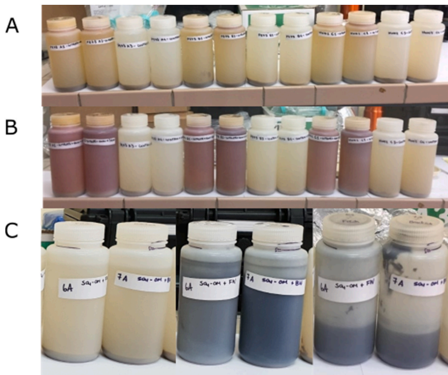
Fig. 4. A: Day 3 \text{FeSO}_4 (10 mM) and \text{NaNO}_3 (10 mM) treatment (first, third and fifth pairs as duplicates) and respective control microcosms (second, fourth and sixth pairs as duplicates, no \text{FeSO}_4 or \text{NaNO}_3 ). B: Day 9 \text{FeSO}_4 (10 mM) and \text{NaNO}_3 (10 mM) treatments showing progressive colour change to red brown (first, third and fifth pairs as duplicates) and respective control microcosms (second, fourth and sixth pairs as duplicates, no \text{FeSO}_4 or \text{NaNO}_3 ) showing no colour change C: Day 9 (left), Day 12 (centre) and Day 34 (right) \text{SO}_4 -lactate (10 mM) microcosm duplicate pairs showing progressive colour change to black. (For interpretation of the references to colour in this figure legend, the reader is referred to the Web version of this article.)
