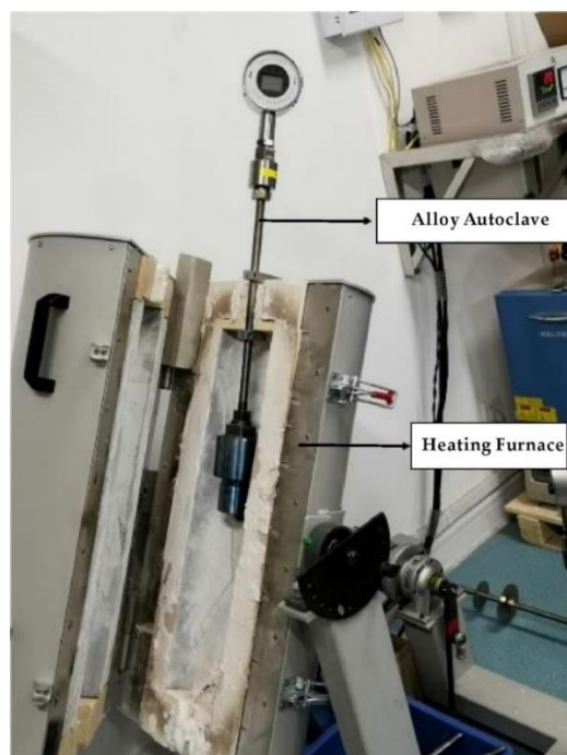
Figure 1. Structural drawing of titanium alloy autoclave.
