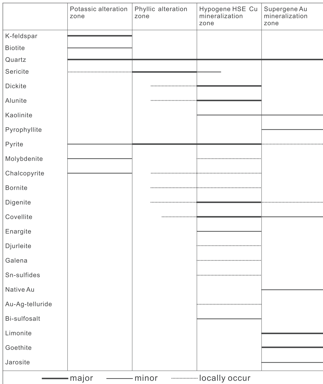
Fig. 3. Paragenetic sequence of ore and gangue minerals from the different alteration and mineralization zones in the Zijinshan deposit.
