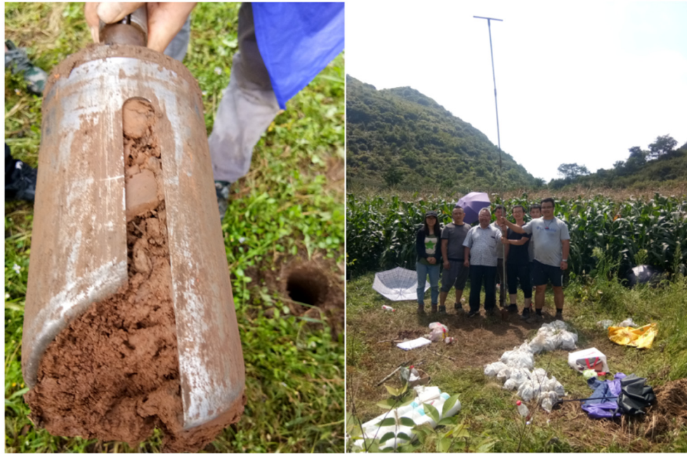
Fig. 5. Auger soil for depth verification.
