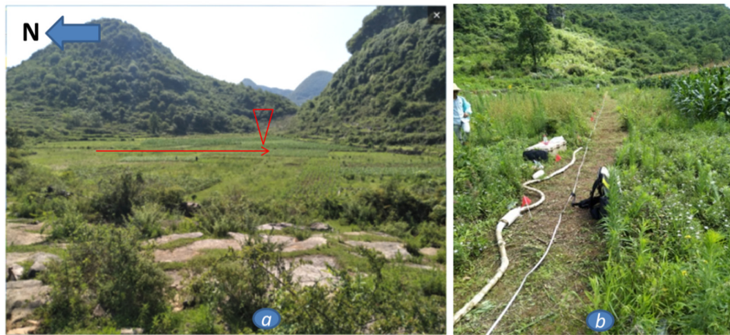
Fig. 4. Photographs of the depression (a) and GPR survey line (b). The red arrow in panel a marks the position of survey line and the red flags in panel b were put every 4 m on the line. The red inverted triangle in panel a marks the position of auger drilling soil.
