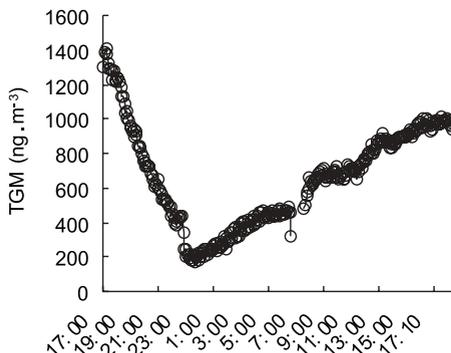
Fig.1 The concentration and trend of TGM in a 6-months landfill vent gas
