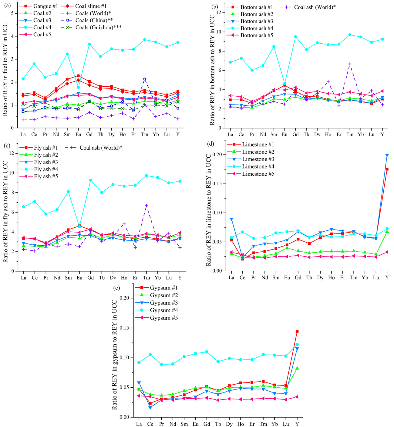
Fig. 5. REY distribution patterns in fuel (a), bottom ash (b), fly ash (c), limestone (d), and gypsum (e) from the five CFPPs (relative to REY in the upper continental crust (UCC) 40 ). * From Ketris and Yudovich 11 ; ** From Dai et al. 14 ; *** From Dai et al. 13
