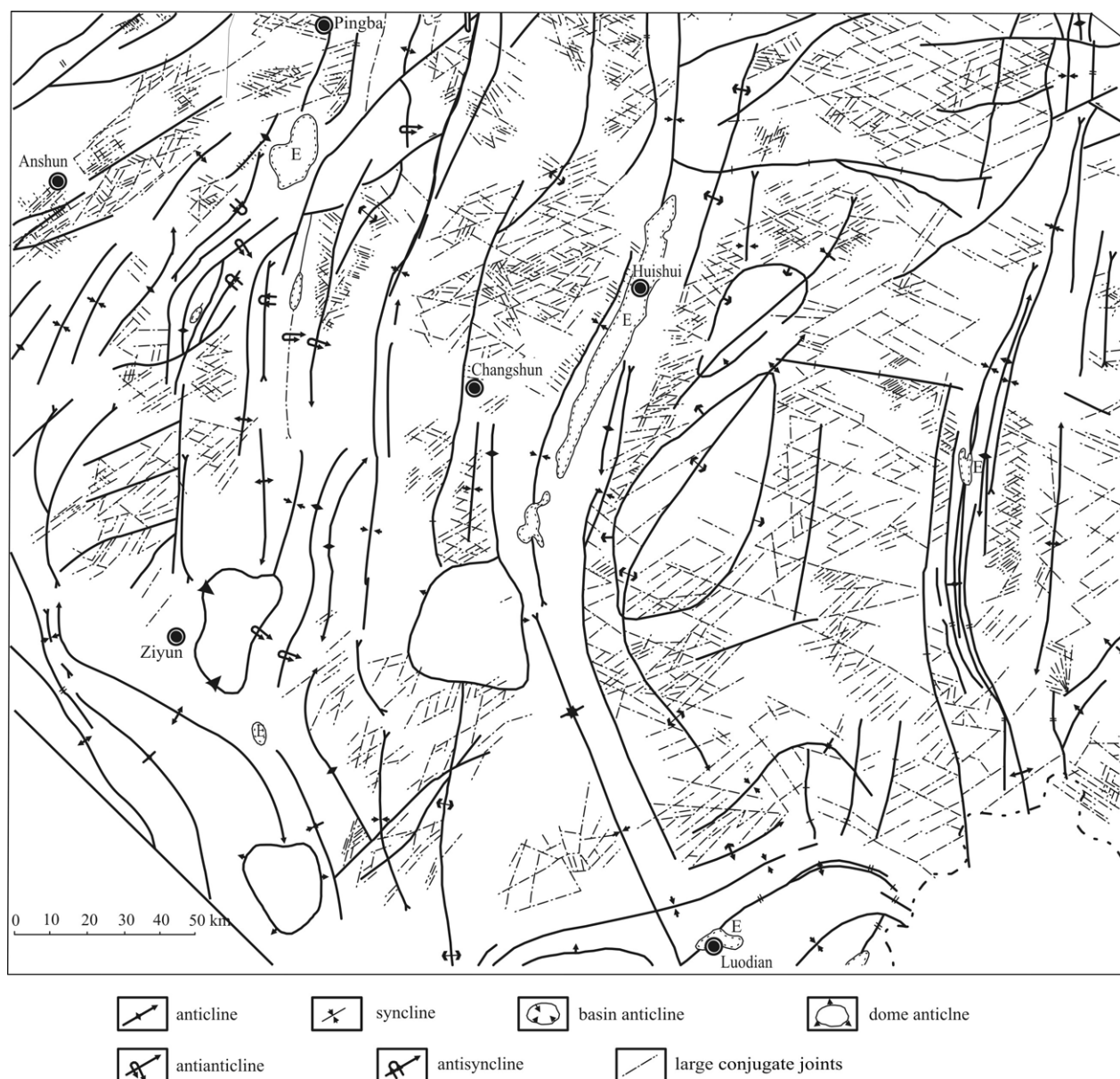
Fig. 2. The distribution of large "X" conjugate joints in the S-N box-shaped folded zones of southern Guizhou (from Gao et al., 1986).
