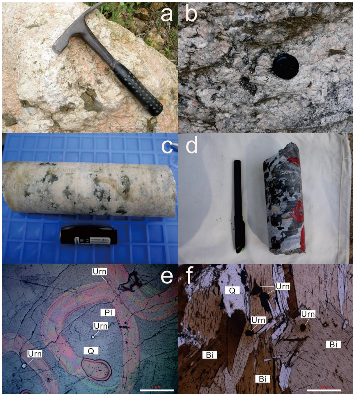
Fig. 3. Images of the biotite pegmatite dikes. (a) Field photograph. (b) Field photograph showing mineralization. (c) Photograph of a representative drill core sample, (d) Photograph of representative drill core sample with plummy biotite aggregations. (e) Photomicrograph of uraninite grains in the quartz and feldspar grains (reflected light). (f) Photomicrograph of uraninite grains in the plummy biotite (transmitted light). Abbreviations are: Bi: biotite; Pl: plagioclase; Q: quartz; Urn: uraninite.
