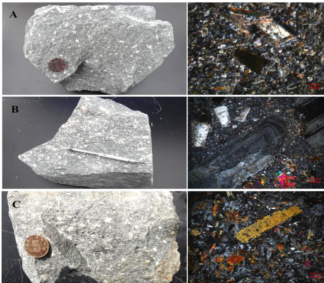
图 2 普朗复式岩体样品照片和显微照片: (A) 石英闪长玢岩、(B) 石英二长斑岩、(C) 闪长玢岩 Fig. 2. Macro- and micro-photographs for samples from the Pulang complex: (A) quartz diorite porphyry, (B) quartz monzonite porphyry, and (C) diorite porphyry.
