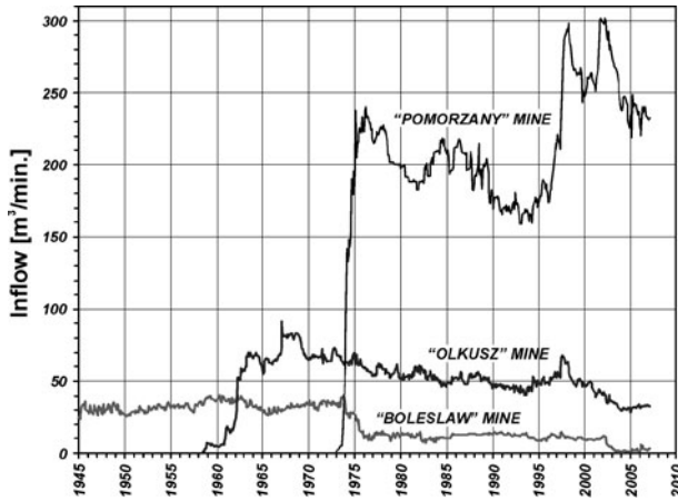
Fig. 2 Groundwater inflows to the Zn-Pb mines in the Olkusz region
