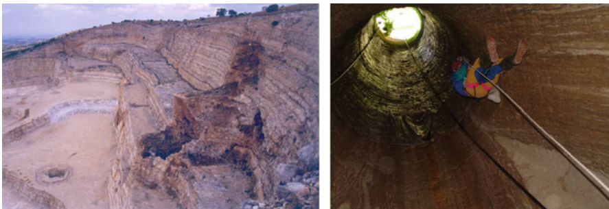
Fig. 5 Surface and underground quarrying: large caves destroyed by quarrying at Minervino Murge ( left ), and an access shaft to underground calcarenite quarry at Cutrofiano ( right )
