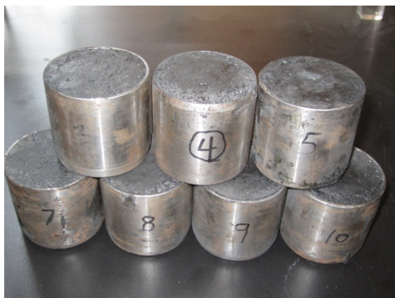
Figure 1 Deformed coal samples used for testing.
