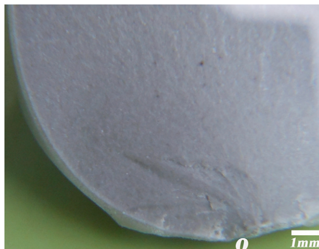
Fig. 5. Representative optical micrograph of fracture surface of the bars. O, origin of the fracture.
