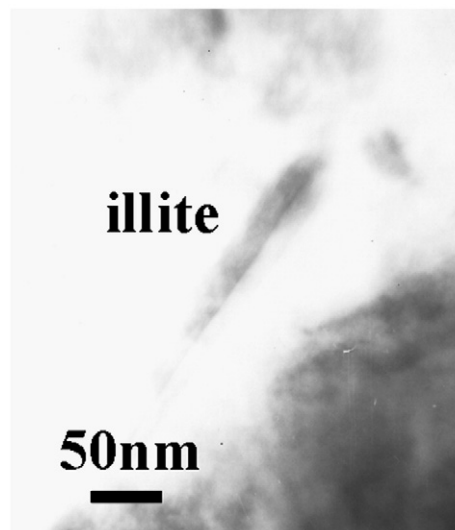
Fig. 13. TEM photomicrograph of illite particle.
