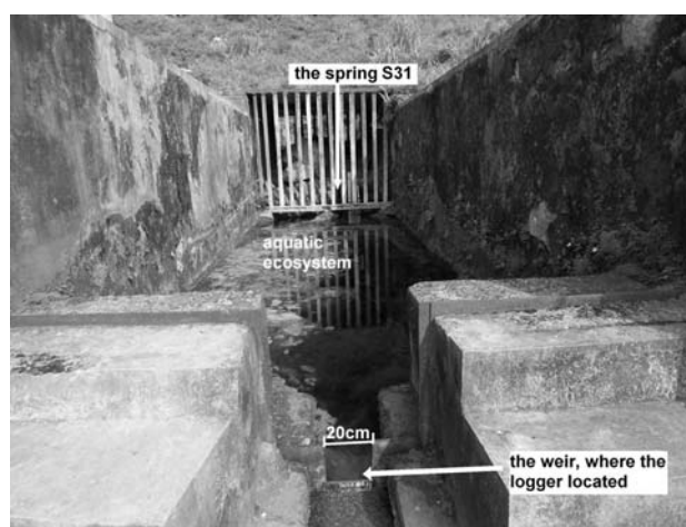
Fig. 1 The spring S31 and the pool with flourishing submerged plants (mainly Spirogyra sp. and Chara Vaillant ex linn ), formed by the weir of the spring, where the data loggers of WTW 350i were located to monitor the variations in physico-chemistry of water. Note that the distance from the spring orifice to the weir is 8.5 m, and some tufa deposits can be found on the aquatic plants' leaves and pool bottom near the weir but not around the spring orifice)
